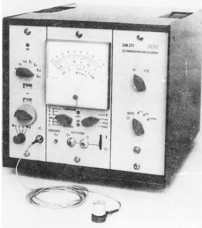
图 2: Vibration meter type 11000 from manufacturer VEB RFT Messelektronik Dresden with accelerometer KD 35, photo from the 1970s. [1]
